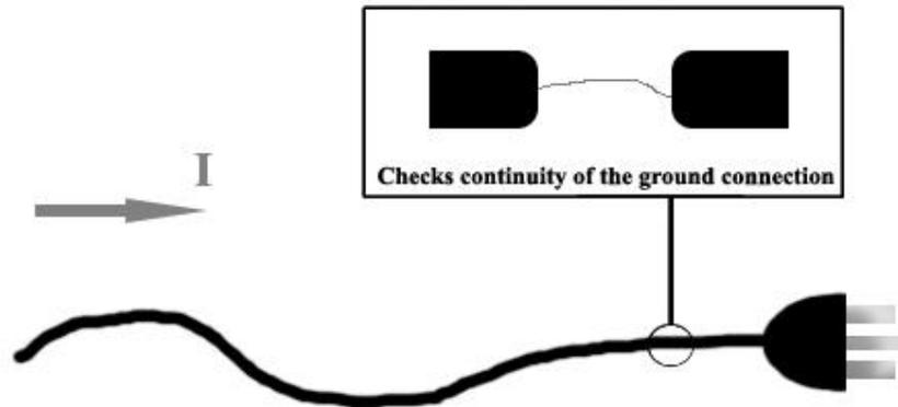
**Figure 1.0: Ground Continuity Test Theory**
