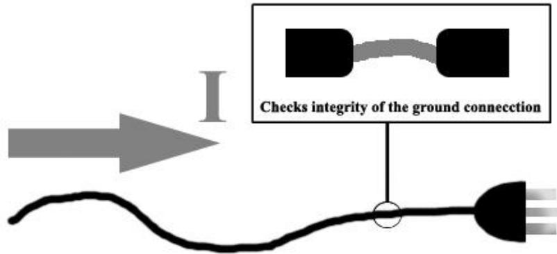
**Figure 2.0: Ground Bond Test Theory**
