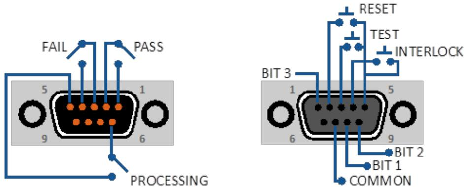
**Figure 2.0: SCI Model 4320 Remote I/O Connectors**
