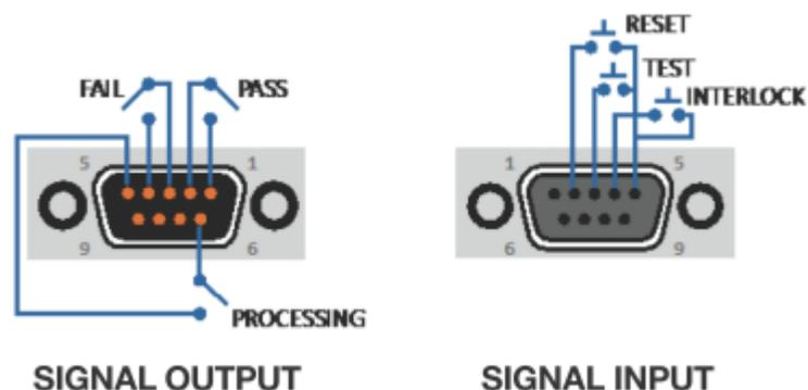
**Figure 1.0: SCI 290 Series Remote I/O pinouts**
